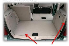
VARIO FLOOR /RAISED - When the Vario Floor System is RAISED it creates underfloor storage and also a LEVEL load area from Tailgate entry across folded
